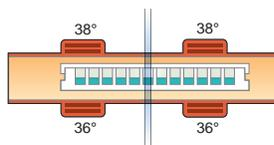
effects typically seen in forced-air systems and the minimal variation across the plate provides consistent assay performance. When lidded or sealed plates are used, the condensation control function prevents interference from excess condensation by setting differential top and bottom temperatures.
