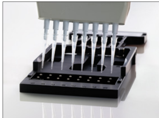
Use the Take3 Micro-Volume Plate with Epoch 2 for direct nucleic acid and protein quantification in multiple 2 µL samples
